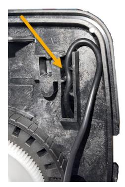
Thread the wire through the strain relief
