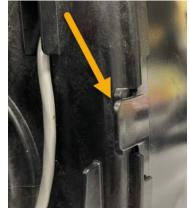
Now remove the drive bracket assembly by pressing up on the drive brackets release tabs and pulling towards you.
