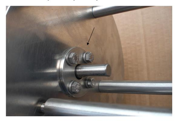
Helping with screwdriver, remove the old gasket and insert the new.
