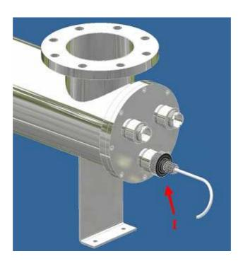
• Mount the o-ring (N) (3043 type) on the probe holder (O) and screw this one on the  $\emptyset$  ¼" bush welded in the middle part of the UV chamber. Finally, connect the pertinente electrical cable.
