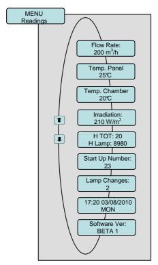
**Flow Rate:** Visible if a flow meter is connected to the UV System. It shows the water flow in m<sup>3</sup>/h passing through the UV system.
