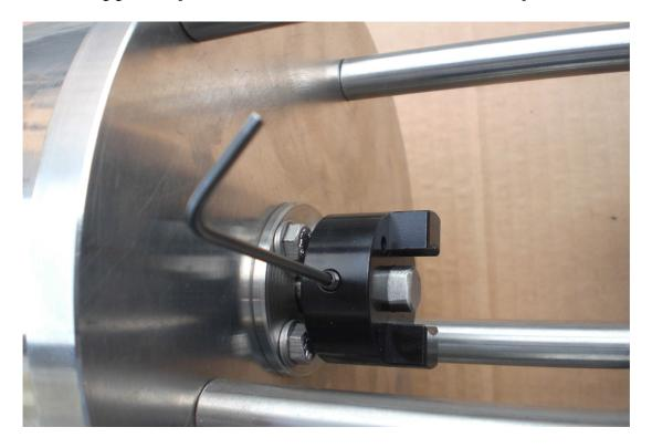
Remove the disc mounted on gasket housing unscrewing its M5 bolts.
