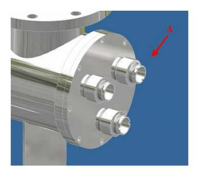
• On the closed side of the UV chamber, mount the blind cap in black polyethylene (D), with the o-ring 2112 type (E) inserted and block by screwing the Ø 1 1/4" ring nuts (F) on the sleeve bolts.
