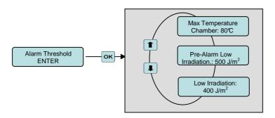
**Max Temperature Chamber:** Visible in case of Rack Plus or SMP systems. This threshold level define the max allowed water temperature in the UV chamber.
