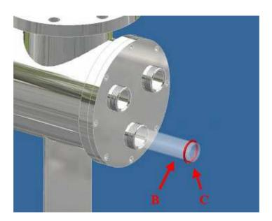
• Screw again the s/s sleeve bolts (A) on both sides of the UV chamber, and carry out the hydraulic test, verifying that the o-rings are watertight and that no water leaks outside the sleeve bolts or inside the quartz sleeves.
