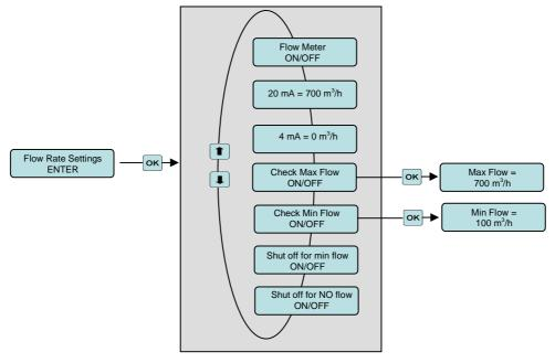
Flow Meter ON/OFF: Set if the flow meter is available.
