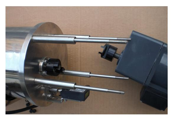
Unscrew the locking grains of joint mounted on the threaded rod and extract the joint.
