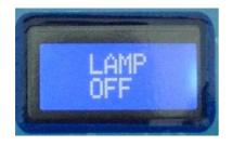
In the case of a non-working lamp. If the system has 2 lamps the failed lamp is identified. Check that the lamp is not broken and/or that the lamp-lighter is working.
