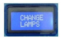
In the case the count-down of lamps-life has come to zero. In such case the lamps must be replaced and the count-down must be started again.
