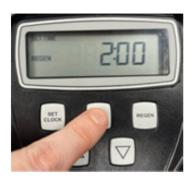
Press **NEXT.** The regen time will appear with the hours flashing. It is set to 2:00am. Use **UP** and **DOWN** arrows to adjust if necessary.
