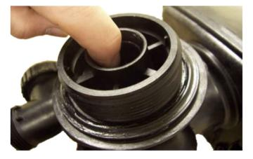
Fit the lower screen to the bottom of the valve. This is a bayonet fitting
