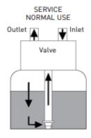
In normal service the water passes through the inlet, down through the resin, up the riser tube to the outlet
