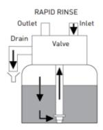
During Rapid rinse water is passed down through the resin and up the riser (same as in service) then to drain. This stage flushes out any residual salt and organics that might be present and re-beds the resin ready for use.
