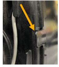
Now remove the drive bracket assembly by pressing up on the drive brackets release tabs and pulling towards you.
