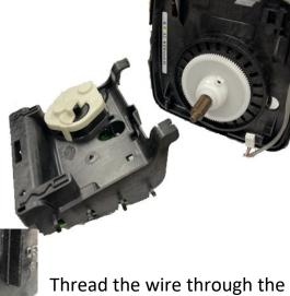
Thread the wire through the hole in the back plate
