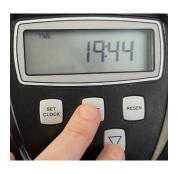
Press **NEXT** and **DOWN** simultaneously for 3 seconds
