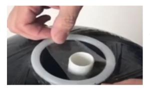
Block the top of the riser tube to stop media getting down the tube. This can be accomplished with tape or a small plastic bag over the end of the tube.
