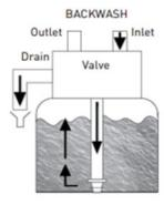
The first stage of regeneration is the backwash. The valve reverses the flow of water so that water now travels down the riser and up through the resin which lifts the bed and loosens any debris that may be trapped in the resin. The water then goes to waste.
