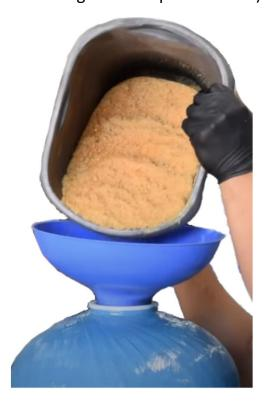
The media can be poured from the bag but we recommend using a smaller container to scoop out the media and pour into the vessel.
