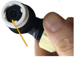
On most of the valves the DLFC is internal but easy to check. Simply pull the red tag on the drain fitting and remove the complete fitting. The DLFC is a small rubber disk with a hole in the centre located on the bottom of the fitting.
