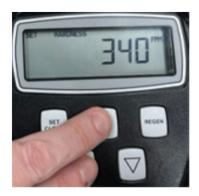
Press NEXT and UP for 3 seconds until "HARDNESS" and 340 appear. Use the UP and DOWN arrows to adjust to your hardness level\* (see notes on page 19)
