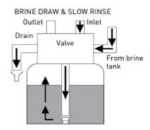
During this stage water is sucked from the brine tank. The concentrated brine is mixed with water from the inlet to reduce the concentration to the correct level. It travels down the riser and up through the resin, when the correct amount of brine has been drawn water from the inlet continues to be drawn up through the resin to push the remaining brine through the resin. This
