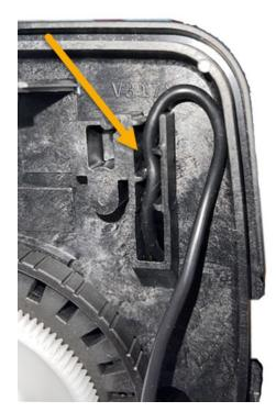
Thread the wire through the strain relief
