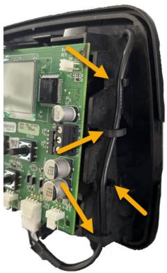
Use the wire guides to hold the wire in position
