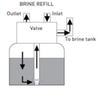
During brine refill a quantity of water sufficient to dissolve the correct amount of salt for the next regeneration is passed through the resin into the brine tank to ensure treated water is used to make the brine for the next regeneration.
