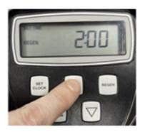
Press **NEXT.** The minutes will now flash. Use **UP** and **DOWN** to adjust if necessary
