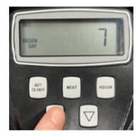
Press NEXT. Regen day will appear use the UP and DOWN arrows to set the regeneration overide day. Eg you can set the softener to regen. every 7 days even if capacity has not been met or it can be set to off.\*\*
