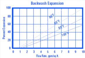
**Backwash:** After each cycle the resin bed should be backwashed at a rate that expands the bed 50 to 75 percent. This will remove any foreign matter and reclassify the bed. The graph above shows the expansion characteristics of Pure PC002 in the sodium form.
