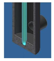
Insert the o-ring Ø 23x4 into the quartz sleeve:
