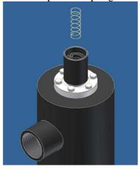
In case of LCD PLUS UV system: Mount the o-ring (3043 type) on the probe holder and screw this one on the  $\emptyset$  ¼" hole in the middle part of the UV chamber. Finally, connect the pertinent electrical cable:
