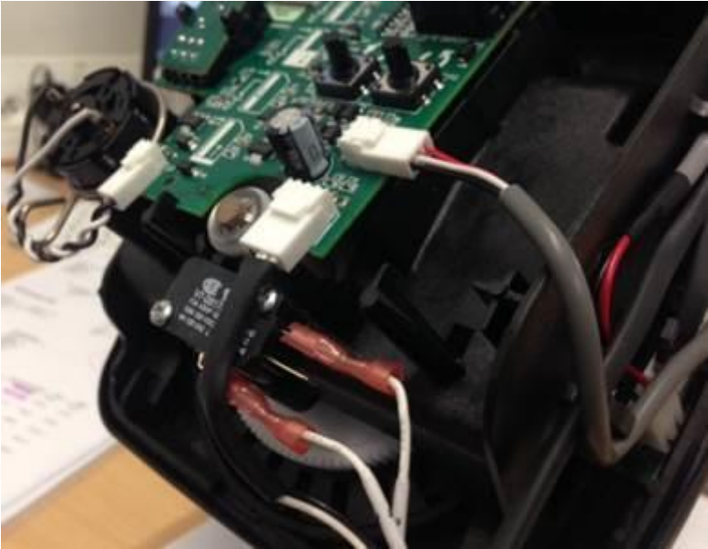
Step 4 Mounting and wiring micro switch side view
